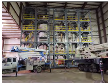
Demonstration autothermal pyrolysis unit at Iowa State University based on RAPID-funded pilot work. Credit: RAPID
