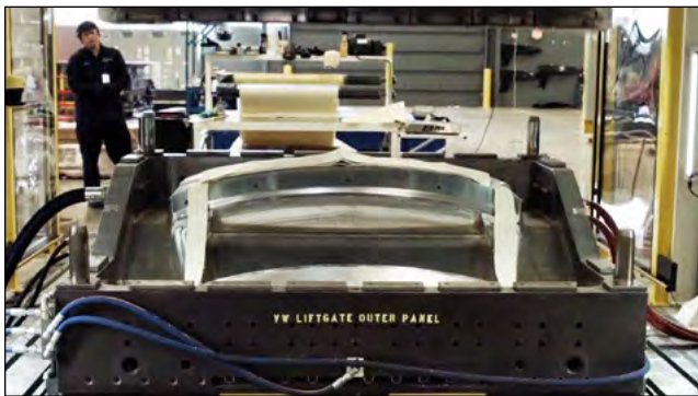
Volkswagenliftgate outer panel on Schuler compression press at IACMI's Scale-up Research Facility in Detroit. Credit: IACMI
